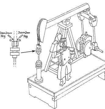
Glue Top Bearing Block to the Beam using 2 diam 3x8 pegs. The end of the Beam which is the shortest distance from the Bearing Block will have the Beam End
