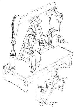
When you have an easy fit at both ends put glue on the base of the Lever Arm Pivot and slide up into contact with the underside of the Top Surface.
