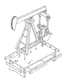
Assemble the balance arm as shown using the usual method of a bead of glue on the back end of each peg. All parts must swing freely like hinges. Note carefully which end has the diam 5mm hole and which end has the diam 3mm. Also make sure you have the slopes in the right position. Slide the diam 3mm hole over the diam 3x115 rod and the diam 5mm hole over the 5x60 rod. These should both be easy fits. You may need to sand the rods to achieve this
