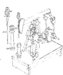
Turn the handle and fully raise the Beam End. Glue a piece of thread in each groove of the Beam End. Lift up the Pump Ro until the Top End Block is just under the lowest end of the Beam End. The ends of the threads are secured in the Top E
