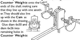
Place small Connecting Rod Ends over diam 6x50 and 6x26 rods.
