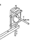
With a little glue in the centres of the main diam 12x5 spacers push onto the shaft on either side of the Bearing Plates: leave a tiny space between the spacer and the Bearing Plate, then glue the
