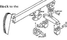
Glue the End Pivot to the centre of the Pull Bar. With a bead of glue on the back end of the diam 5x20 peg, push through the End Pivot and Short Bearing Block. This should
